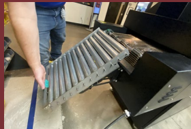
Adjustable rate conveyor system
